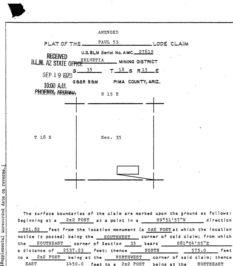
notice is posted) being the <u>SOUTHWEST</u> corner of said claim; from which the <u>SOUTHEAST</u> corner of Section <u>35</u> bears <u>S81°04'05"E</u> a distance of <u>2537.23</u> feet; thence <u>NORTH</u> <u>575.0</u> feet to a 2x2 POST being at the NORTHWEST corner of said claim; thence 1450.0 feet to a 2x2 POST being at the NORTHEAST EAST corner of said claim; thence SOUTH 575.0 feet to a 2x2 POST being at the SOUTHEAST corner of said claim; thence WEST 1450.0 feet to the place of beginning.
